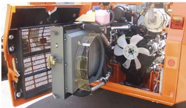
Fig. 2. View of the combined cooler open
